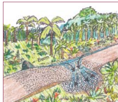
Figure 6.2. Wide dips allow ditch runoff to be directed by berms to flow across road to stable outlet. Not for use on grades greater than 12% (Adapted from: Wisconsin Department of Natural Resources).
