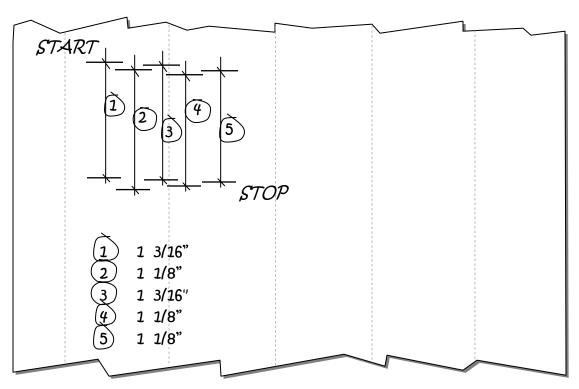
Figure 6.15: Example of how to mark & notate level markings using the "Falling Head" percolation test method, where the hole is re-filled to 6 inches between every measurement interval.
