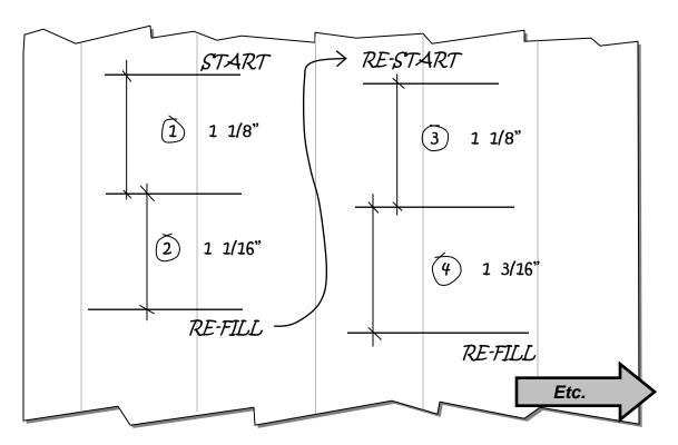
Figure 6.14: Example of how to mark & notate a re-fill during the percolation test.
