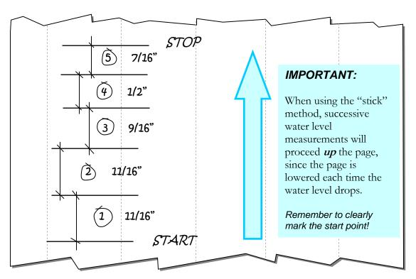
Figure 6.13: Example of how to mark & notate level markings using the removable measurement form. Level readings are marked as horizontal pencil marks, vertical measurement lines are drawn later to assist with measurement. Interval numbers and measurements are written in by hand.
