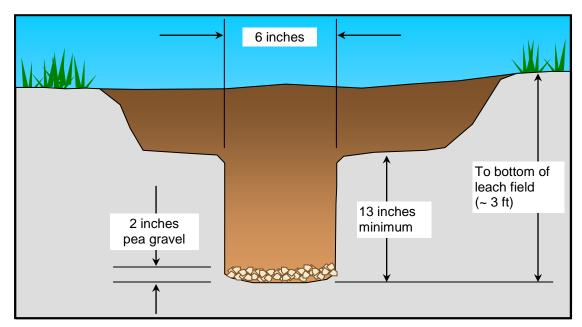
Figure 6.5: Standard percolation test pit dimensions
