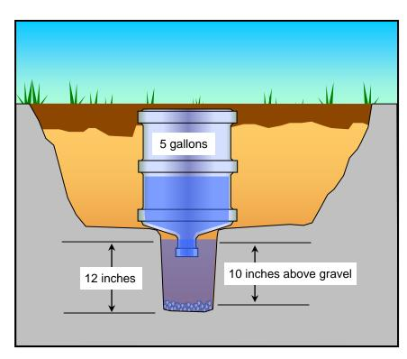
Figure 6.9: Inverting a 5gallon water bottle over the hole is a good way to maintain the 12-inches required depth while the hole remains unattended, for example, overnight. Just make sure the bottle is securely supported so that it doesn't fall down and spill the remaining contents. Also, be careful not to scour the bottom or sides of the hole while filling in this manner. Once the bottle is inverted, the water in the hole will remain calm, just like in an office or home water dispenser.
