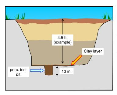
Fig. 6.8: A clay layer is found at 5 feet in the deep observation hole. Because this would be within 3 feet of the bottom of the leaching field, the percolation test must be conducted within the clay layer; NOT the overlying, more permeable soils.
