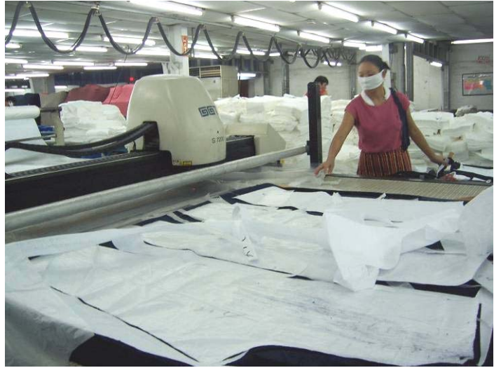
Saipan garment factories perform both manual cutting (left) and automated cutting systems (above).
